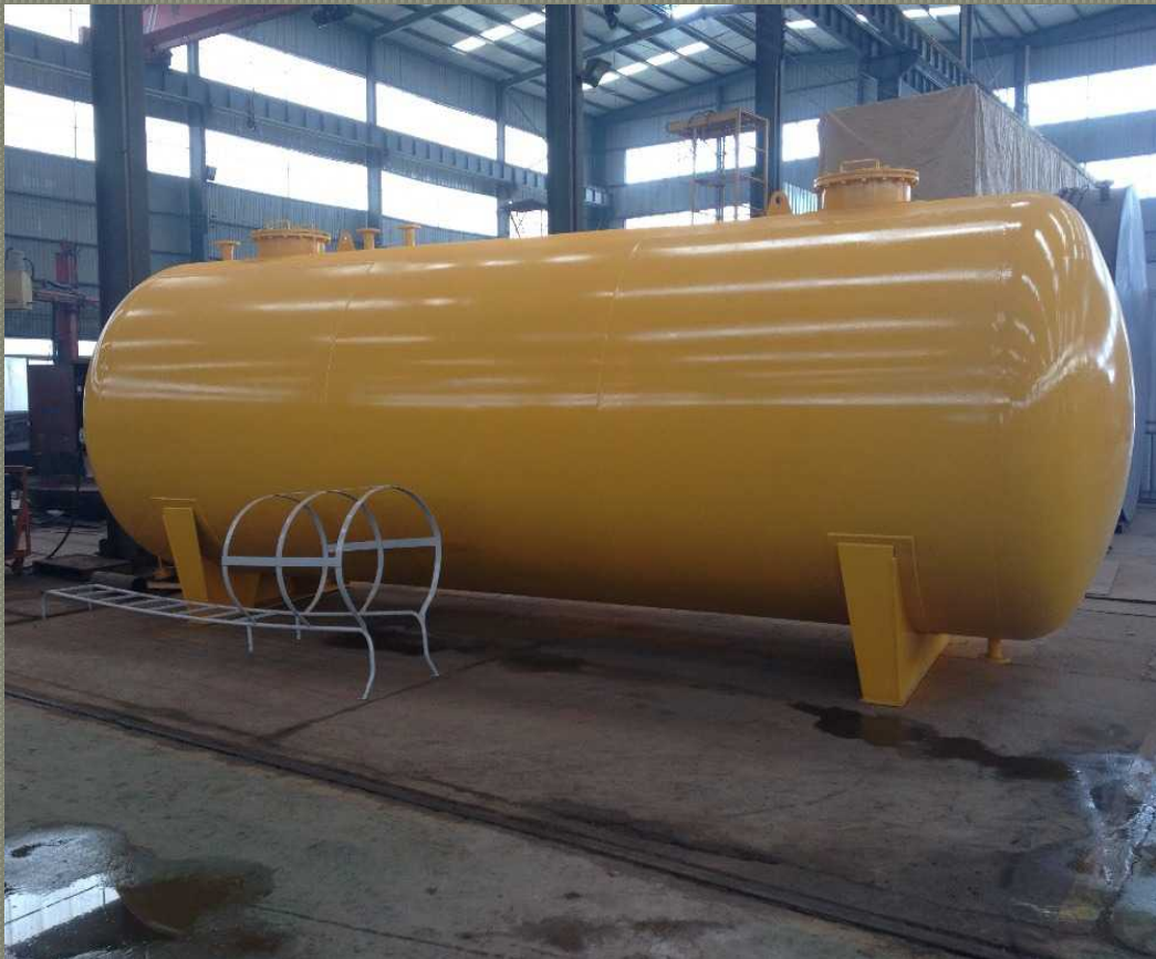
Cylindrical Tank for Caterpillar generator
